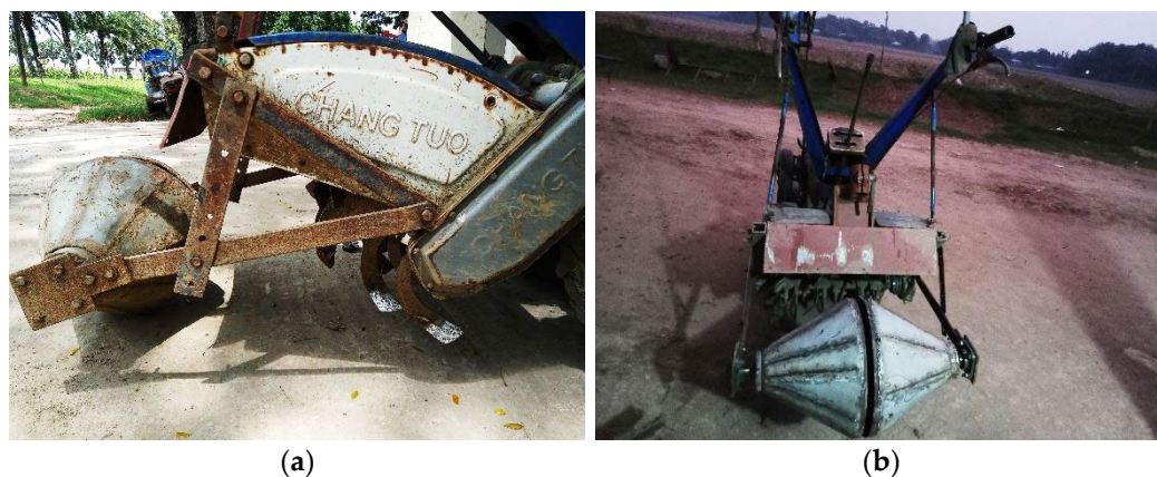
Figure 9. Developed earthing-up machine. (a) Side view of earthing-up tool. (b) Rear view of earthing-up machine.
