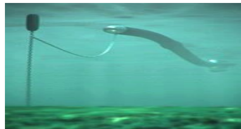
Image of the anaconda bulge wave power device
