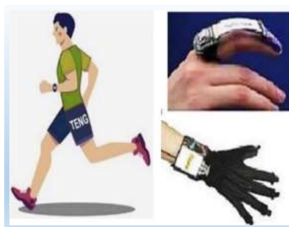
Fig. 8. MXene-based TENG mounted on different parts of the body for harvesting energy from human muscle movements and from feet pressure.
