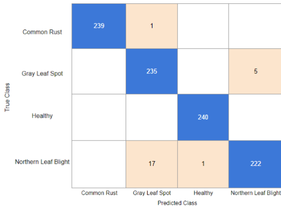
Fig. 9. Confusion matrix of corn dataset using pre-trained ResNet-101 model, with TP, TN, FP, and FN values.
